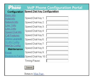
Fig 5: Configuration of Speed Dial Keys
